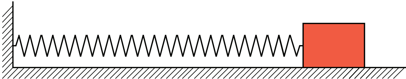
Mass point on a spring (with no friction)
